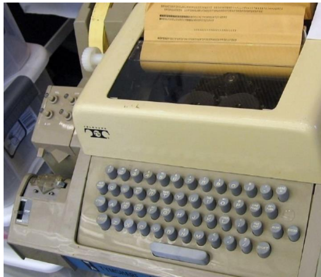
Figure 2 Teletype Model 33, a widely used teletype used as a computer terminal.
